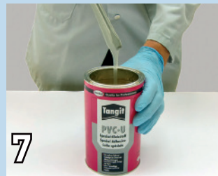
7 Stir solvent cement thoroughly and check consistency
