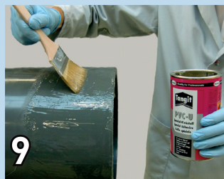
9 Apply solvent cement in the middle of the pipe cementing surface & distribute it first radially than axially all over (2 people)
