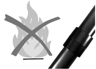
No open flames when cementing. No smoking.
