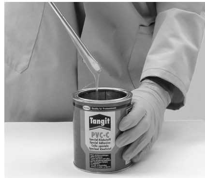
Checking the cement
