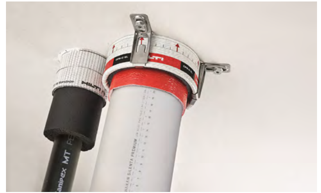
Zero distance to pipe systems such as GF Sanipex MT with flammable Synthetic rubber insulation (Armaflex, Insul-Tube, Kaiflex...) and Hilti Firestop bandage CFS-B for heating or drinking water applications
