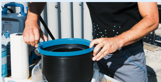
Place the mounting aid on the fitting. Stretch the sealing lip pressing the handles together.
